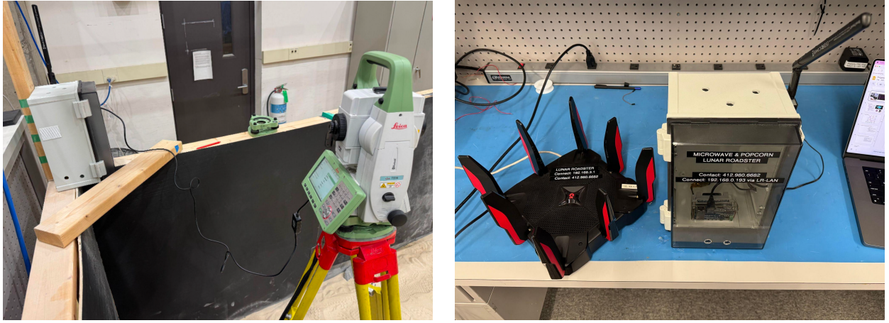
Figure 8: Left, Leica TS16 Total Station connected to TX2 Relay. Right, LAN Router and NVIDIA TX2 Relay
