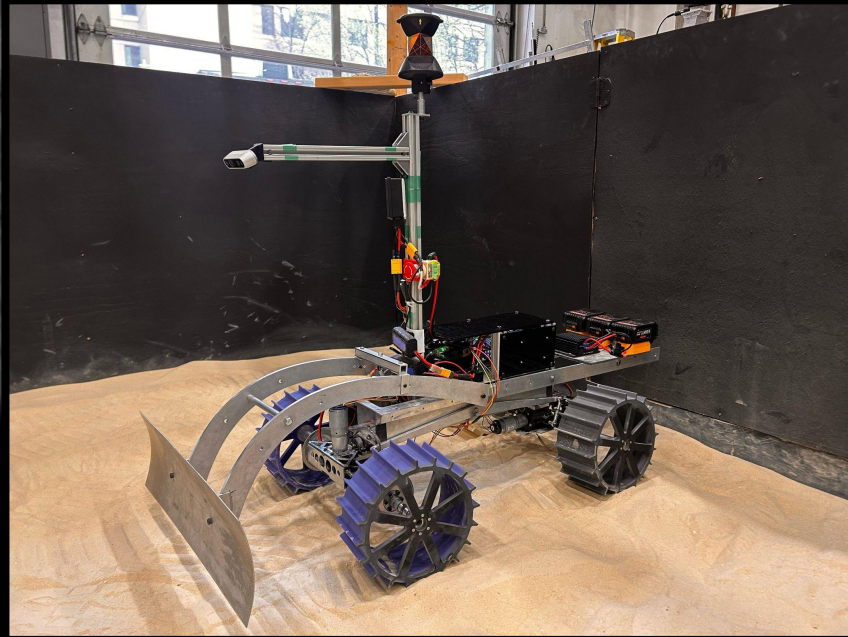
An autonomous mechatronic bulldozer for the Moon
